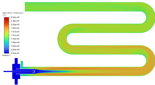
Fig. 2 Temperature contour at the central cross-section of the radiant tube burner (100 % CH 4 with 10% excess air).
